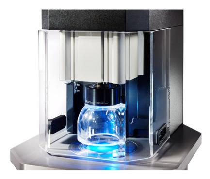
Replace the raised insert with the corresponding one to the chosen test dome.
