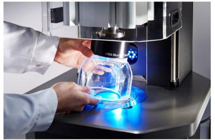
Remove the test dome from the end of the clamp piston by carefully pulling downwards; the dome is held secure by magnetic force.
