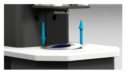
With the test dome removed, the stainless steel clamp ring can be removed by pressing on the top surface close to the outer edge. The clamp ring will lift up at the opposite edge.
