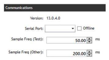
When not testing, the data collection frequency is reduced to 200 ms (5 times per second), mainly to observe the status of the Titan instrument.
