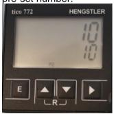
The Pre-set Counter can be reset to zero by pressing the Up and Down keys together, as indicated in the picture below
