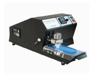
CrockMaster Motor Driven Crockmeter Model 680
