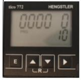
Use the right-arrow key again to move by one position to the right. Then use the Up or Down key to increment or decrement the position by 1.
