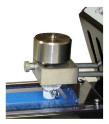
Cover the finger with the undyed crocking cloth and secure in position with the spring clip provided, making sure that the spring clip is clear of the specimen clamp. Lower the head arrangement onto the rubbing area, reset the counter using the "RST" push button located on the face and commence the straight line motion pressing the green start button. The digital counter will increment one digit for each completed cycle.
