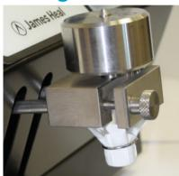
The rubbing finger can be removed by turning the "clamp screw" anti-clockwise until the clamping pressure is released. Replace the rubbing finger. Apply clamping pressure to secure the finger by turning the clamp screw clockwise.
