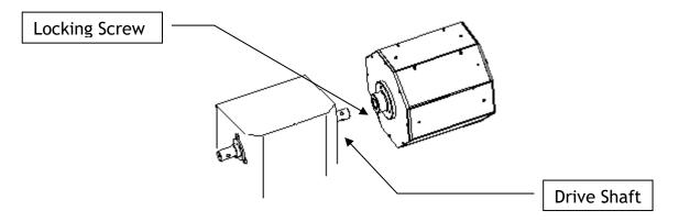
SnagPod can be removed simply by fully unscrewing the locking screws using the 4mm hexagon key. When the screws are fully retracted, carefully slide the box off the end of the shaft. Ensure both drive shaft and mounting flange are clean before reassembly.
