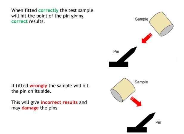
If the SnagPod has been used incorrectly inspect the pins for damage and change them if required.
