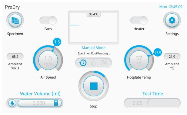
13. The specimen will equilibrate for 5 minutes, after which time the user is notified by an audio signal and blue flashing lights that the water can be applied to the Hotplate.
