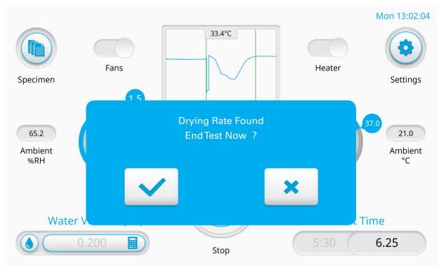
You can choose to end the test when the drying rate has been detected automatically by pressing the tick, alternatively press the cross icon to extend the test time.
