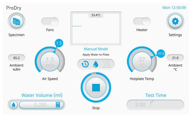
14. Open the lid and lift the free end of the Specimen; apply the water to the centre of the Hotplate using a Micropipette.
