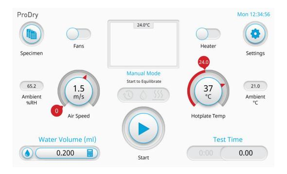
The following sections describe the operation and data analysis for ProDry testing in accordance with AATCC - 201 Drying Rate of Fabrics: Heated Plate Method.
