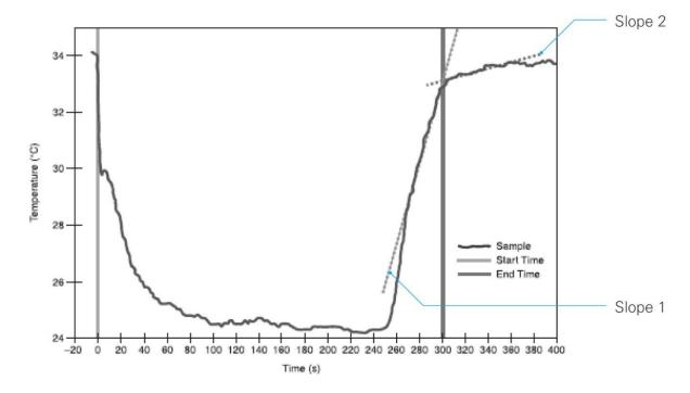
The ProDry software is able to analyse the temperature plot during a test and automatically calculate the Test End Time and Drying Rate.
