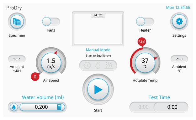
2. Press the Fans and Hotplate toggle buttons on the touchscreen to activate them (they will automatically default to the values specified in the AATCC Test Method 201.) Toggle the fan and heater switches and wait for the air speed and hotplate temperature to reach values specified.
