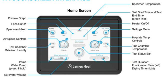
**Graph:** Automatically plots the data as it is recorded providing immediate visual feedback on current test.
