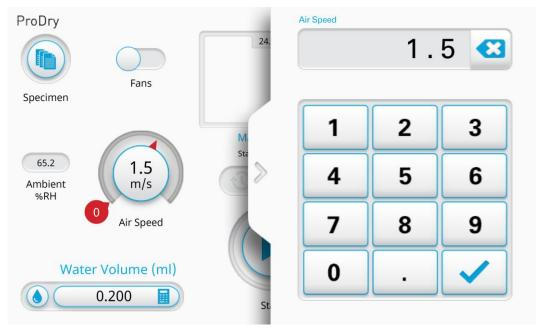
**Ambient %RH:** Displays the test chambers relative humidity.
