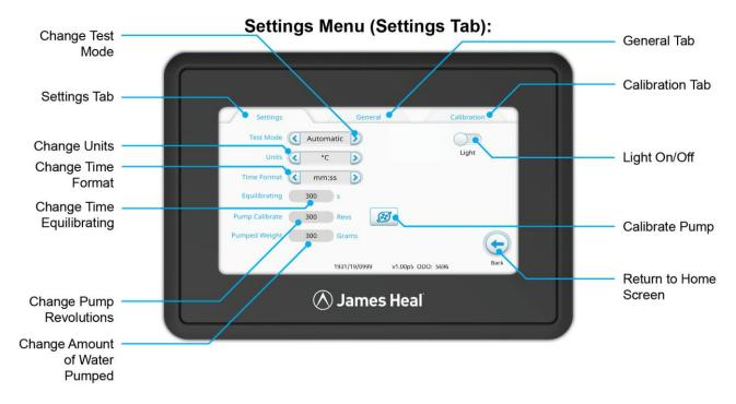
Test Mode: Change test mode between Automatic and Manual Dosing.
