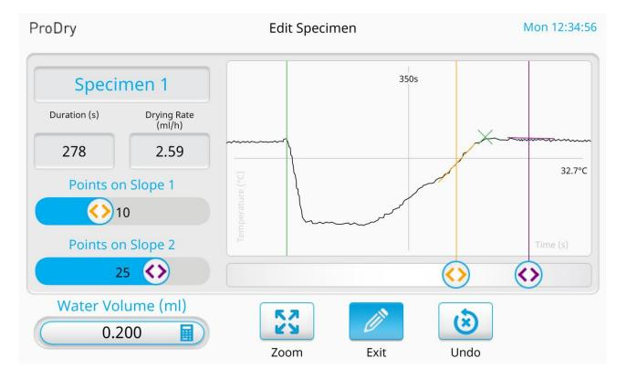
The user can decide to save these alterations or undo any change and revert back to the automatically calculated result.
