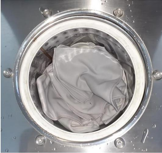
Balance the fabric load evenly within the spin dryer drum - failure to do so will cause imbalance and excessive wear on the machine.
