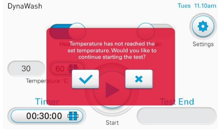
If the start button is pressed to start the test before the bath temperature has reached the set temperature, a warning message is displayed. This is only applicable when the heater toggle is on.
