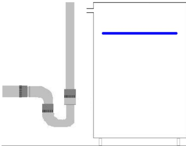
At the rear of the bath is a 22mm drain connection for emptying via the pump. Connect the hose and clamp and ensure that the drain pipe is higher than the water level in the bath to prevent the water siphoning from the bath.
