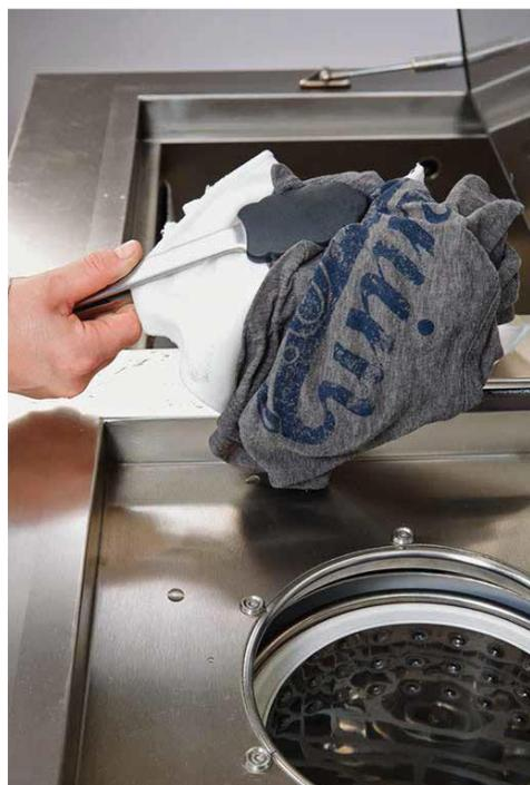
At the end of the tests, the specimens and makeweights may require spinning in the spin dryer.
