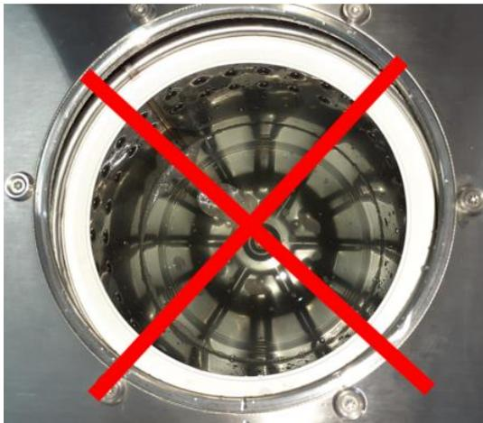
Never fill the spin dryer with water alone, there must always be a fabric load present.
