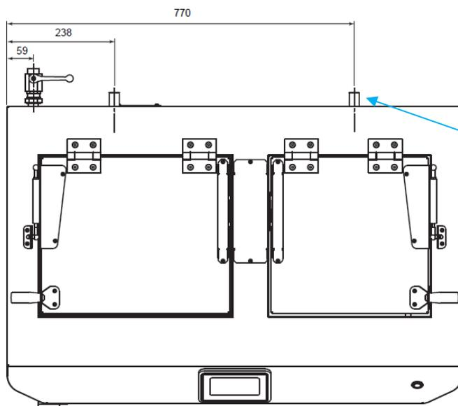
DynaWash Duo has a second 22mm drain connection for carrying away the excess water from the spin dryer.
