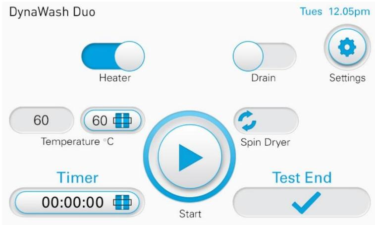
Once the test is complete, the test end will display a tick, the timer will display all zeros and the progress ring will be complete. The heater and impeller stop.
