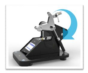
Remove any weights from the pendulum. Release the pendulum & hold in the position shown in the picture on the left. Please take care when doing this.
