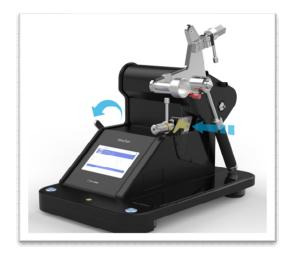
Raise the blade by using the blade handle on the left hand side of the instrument. Remove the blade by loosening the screws, and replace with a new blade.
