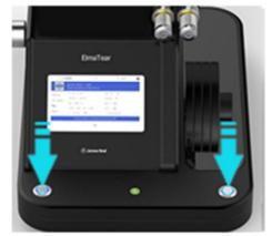
Please press both buttons at the same time to release the pendulum.
