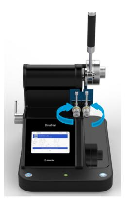
Place a test specimen centrally in the jaws so that the specimen is set carefully against the bottom of the jaws.
