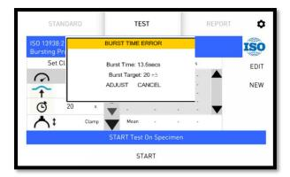
ISO 13938:2 requires the time to burst to be  $20 \pm 5$  seconds. If the first test is not with in the correct time an error message will appear on the screen.
