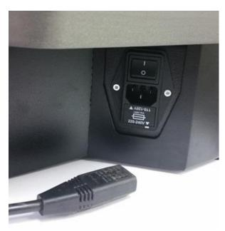
Two (2) fuses are fitted, located at the rear of the machine beneath the mains lead socket.
