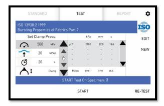
The instrument will automatically stop if it detects a burst and will display the final test result.
