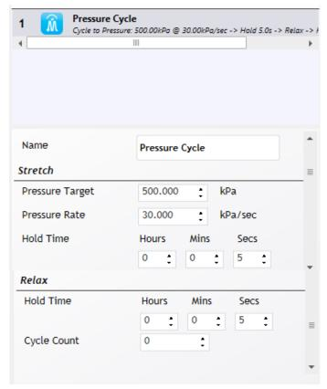
For cyclic testing to a known pressure, select **Pressure Cycle** to set the **Stretch**:
