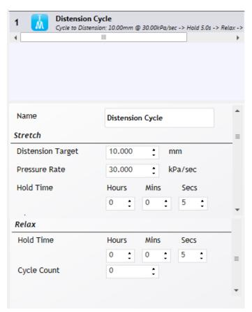
For cyclic testing to a known distension, select **Distension Cycle** to set the **Stretch**:
