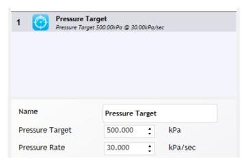
Set the required **Pressure Target** and **Pressure Rate**.
