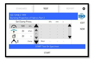
The **TEST** screen shows live data and stores each result temporarily.
