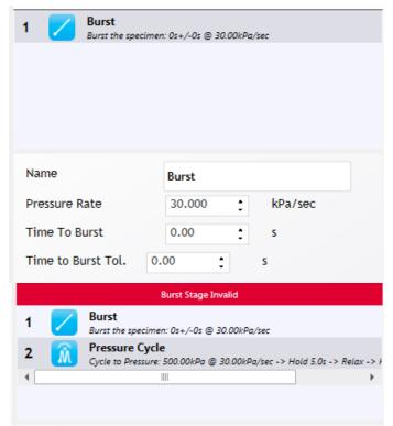
The burst parameters can be altered once the **Burst** stage has been selected:
