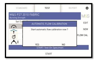
Before testing can commence, the flow needs to be calibrated.
